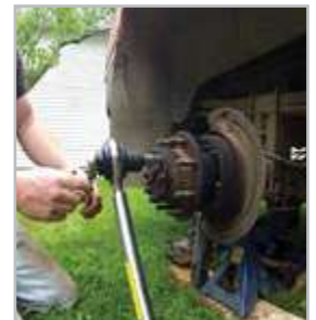
Torque multiplier used for lug nuts
