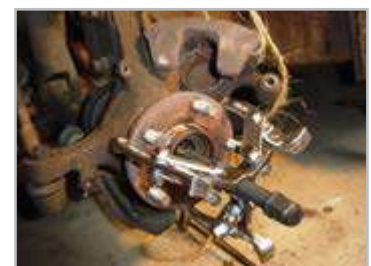
3 Jaw Puller used for removing tyre hub
