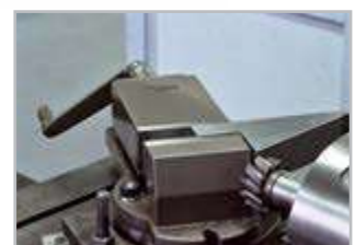
Milling Machine Vice being used to hold a job for milling operation
