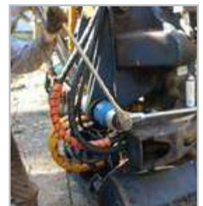
Torque multiplier used for machine nut tightening
