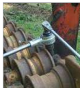
Torque multiplier used on tracks
