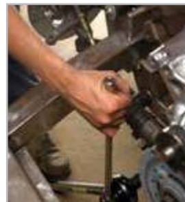
Torque multiplier used in inaccessible areas
